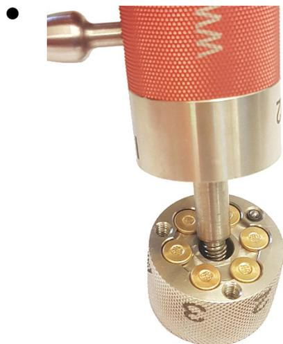
Hold the filled drum with one hand and guide the axis of the main unit through the drum with the other hand.
