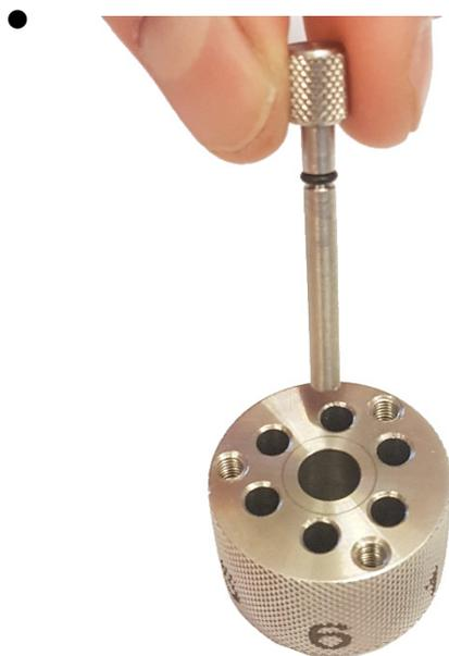
Remove the cartridges or empty shell casings from the drum. If necessary, use the ejector to eject the shell cases from the front of the drum.
