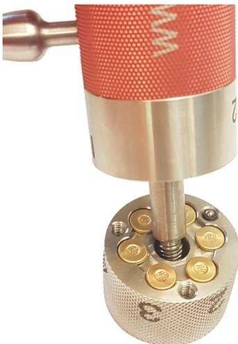
Hold the filled drum with one hand and guide the axis of the main unit through the drum with the other hand.
