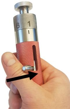
Use your thumb to push the cocking lever to the right until it jumps out of the locking position and fires the cartridge.
